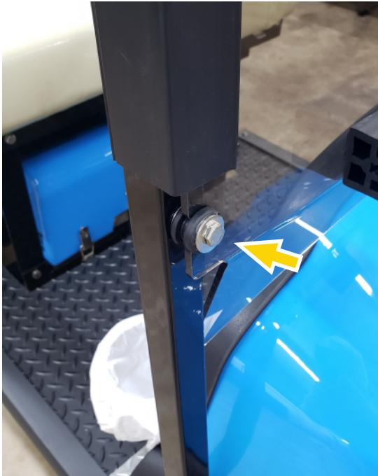
8. Install the vinyl top with the round pocket and 2 nylon loops towards the front of the cart. Slide the pocket over the front of the frame and affix the nylon loops to the posts on the underside of the top frame. In the rear, pull the vinyl top over each corner and affix the nylon loops to the posts on each rear vertical rail. Do not forcefully pull the loops. If there is too much slack in the loop, twist or tie the knot in the middle.
