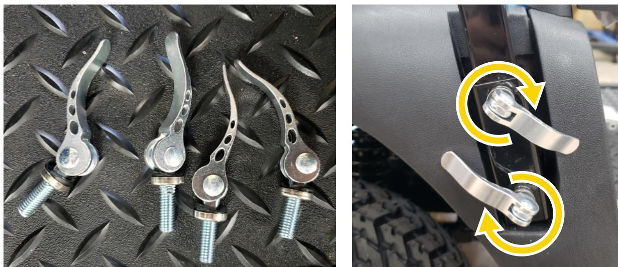
3. Loosen the thumb knobs on either side of the rear basket, insert the rear vertical rail with the bend facing forward on both sides, and leave the thumb screws loose. The frame should look like the image on the right at this point:
