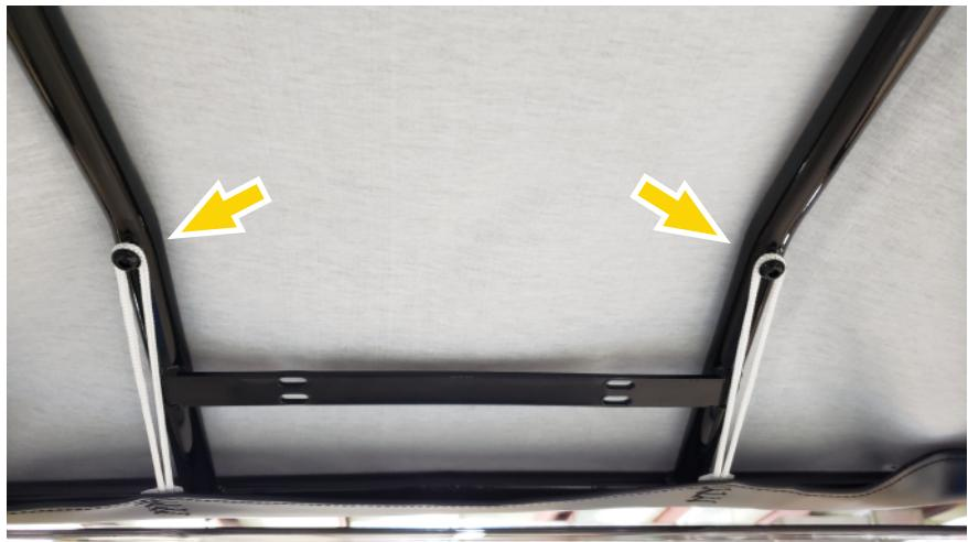
9. Insert the black rubber rail end plugs into the top end of the four rails.
