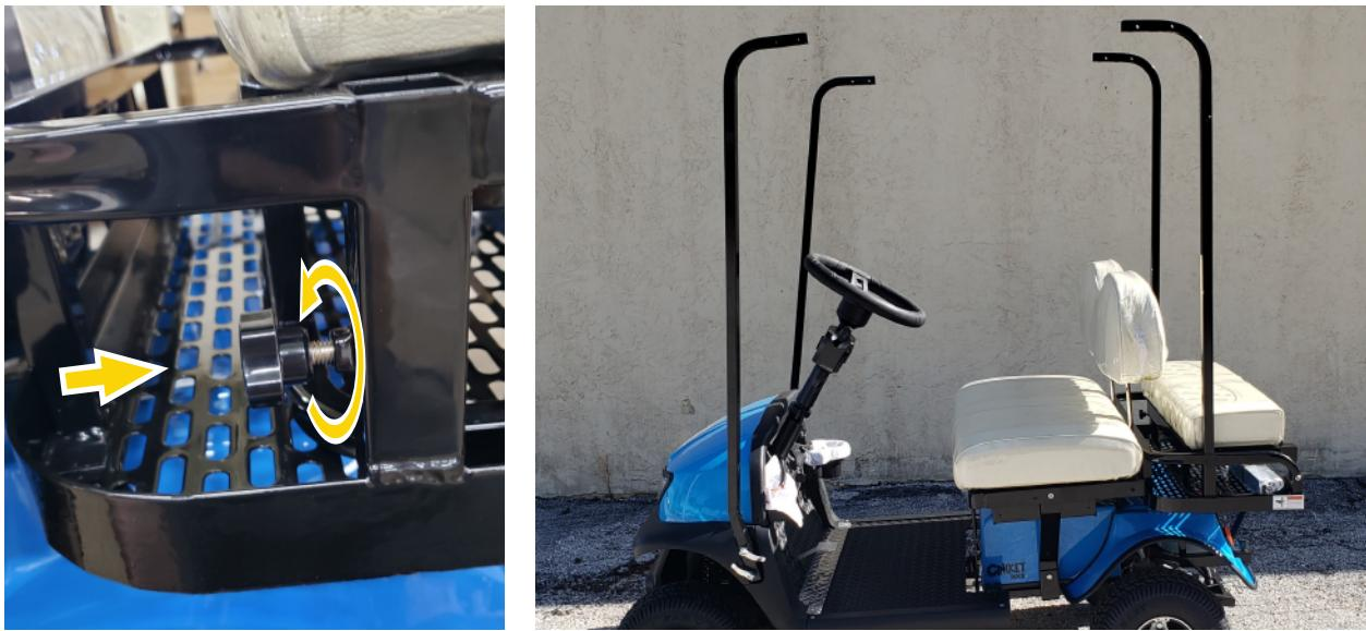
4. With the rear view mirror mount on the top frame facing the front of the cart, loosely fasten the four short bolts with a washer on either side into the four holes on the rear part of the frame with the nylock nuts. Do the same with the four long bolts on the front, but be sure to place the black spacer between the vertical bar and the top frame as pictured below.
