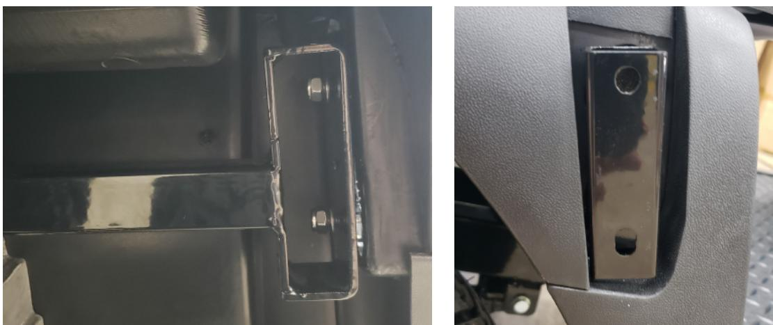
2. Slot the vertical rails with the slight bend at the base into the quick release brackets. After placing the plastic and metal gromet on the quick release bolts with the plastic facing the lever, screw the bolts through the quick release bracket into the bent vertical bar. Use the lever to secure the quick release.
