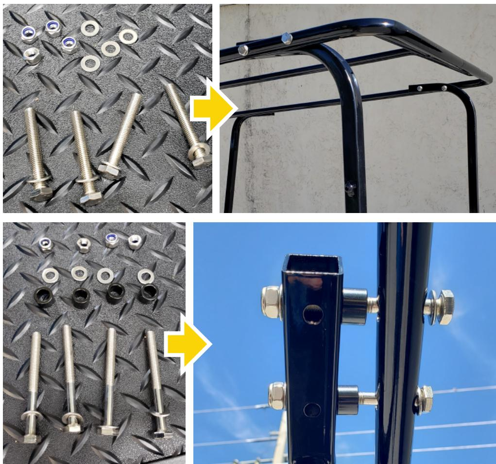
5. With all of the top frame bolts in place, tighten all of them using a 14mm socket or wrench on the bolts and a 13mm socket or wrench on the nylock nuts. Be sure to tighten up the nylock nuts on the quick release bracket posts as well.
