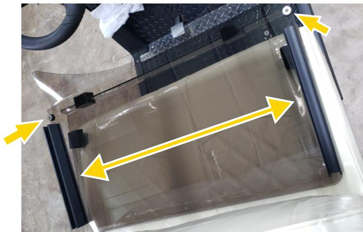
7. Align the black plastic clips with the front vertical rail and snap them into place. Slide the windshield up or down until the hole in the rubber grommet matches the hole in the front vertical rail. Insert the bolt and tighten the hardware down using a 10mm wrench or socket. With the windshield installed, you may remove the protective film if you have not already.
