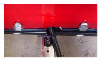
c. Then push T-handle back down securely to lock vehicle in preferred position.
