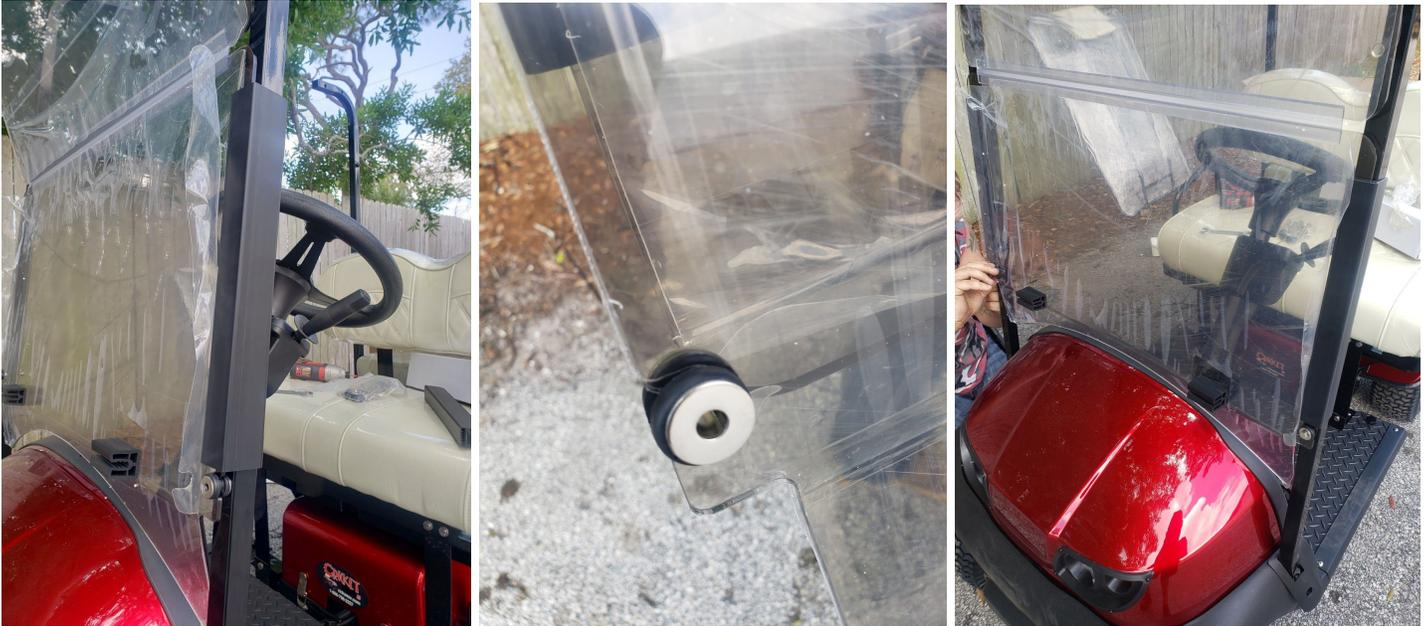
6. Slide windshield up or down until the hole in the rubber grommet matches hole in front vertical rail. Install & tighten this hardware as shown below. Do this to both sides.
