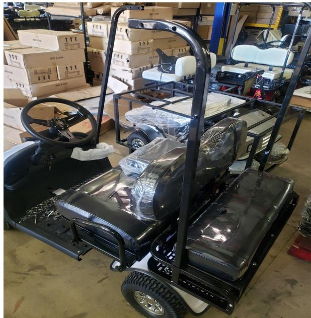
4. Install front rail cover by sliding down from the top of rail as show in picture below to both sides.
