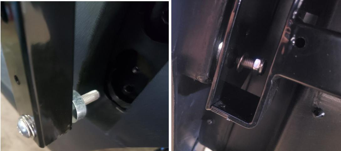
2. Do the same with the top hole. Leaning back rail may make it easier to install spacer. Repeat step 1. & 2. to the other side.
