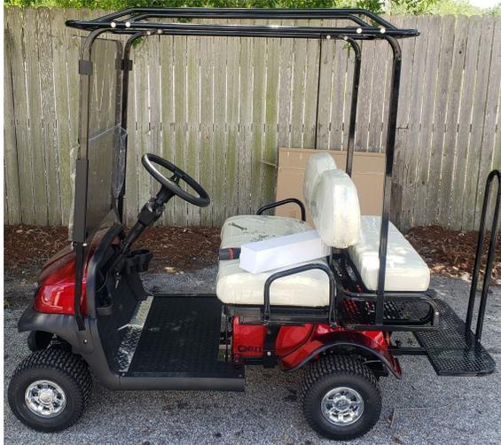
1. Install front vertical rail with slight bend at the bottom and roughly 90 degree bend facing toward the back of the cart. Starting with bottom hole Loosely attach hardware shown below. Start with bottom hole first.
